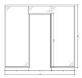
The declared system consists of two 12.8 mm thick laminated single layer glazed elements measuring 2400 x 900 mm, and a door opening measuring 2100 mm x 900 with glazed panel above the door opening. The full DEKO FG partition system including door opening is 2700 mm wide and 2400 mm high, equivalent to 6.48 sqm. Excluding door opening, the FG partition system totals 4.59 sqm.
